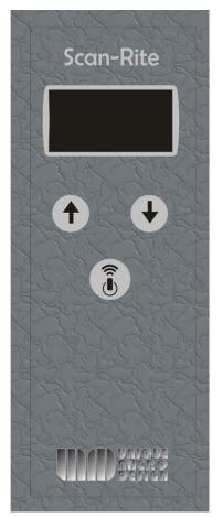
The Unique Micro Design Scan-Rite<sup>TM</sup> Model 641A-02 is a portable hand held RFID microchip reader that has been specifically configured to meet the needs of the equine industry to confirm the identity of microchipped horses.
