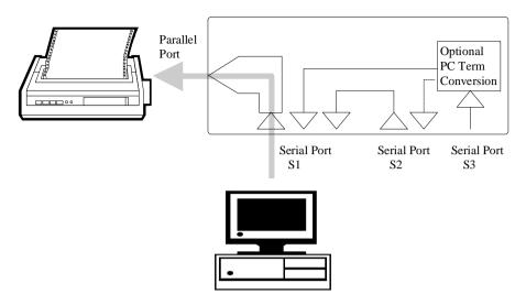
As *Mode 2* has input from serial port S2 directed to S1, a host computer could communicate with a parallel printer whilst receiving input from a bar code scanner.
