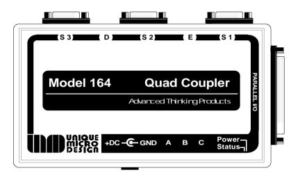
The three serial ports on the *Model 164* are designated *S1*, *S2* and *S3*. A parallel port is also provided which can be configured either as an input, designated *PI*, or configured as an output, designated *PO*.
